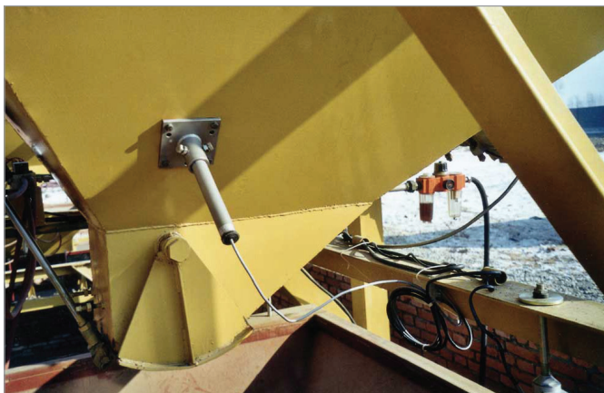
External fixing of a probe at the funnel
